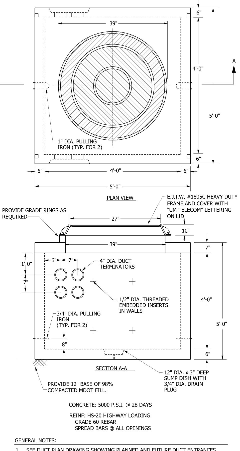
1. SEE DUCT PLAN DRAWING SHOWING PLANNED AND FUTURE DUCT ENTRANCES, ON CURRENTLY PLANNED DUCTS , PROVIDE TERMINATORS AT LOCATIONS SHOWN, TERMINATOR LOCATIONS SHOWN IN DETAIL ARE EXAMPLES. FOR FUTURE DUCT RUNS PROVIDE KNOCKOUTS SIZED AND LOCATED AS NOTED.
